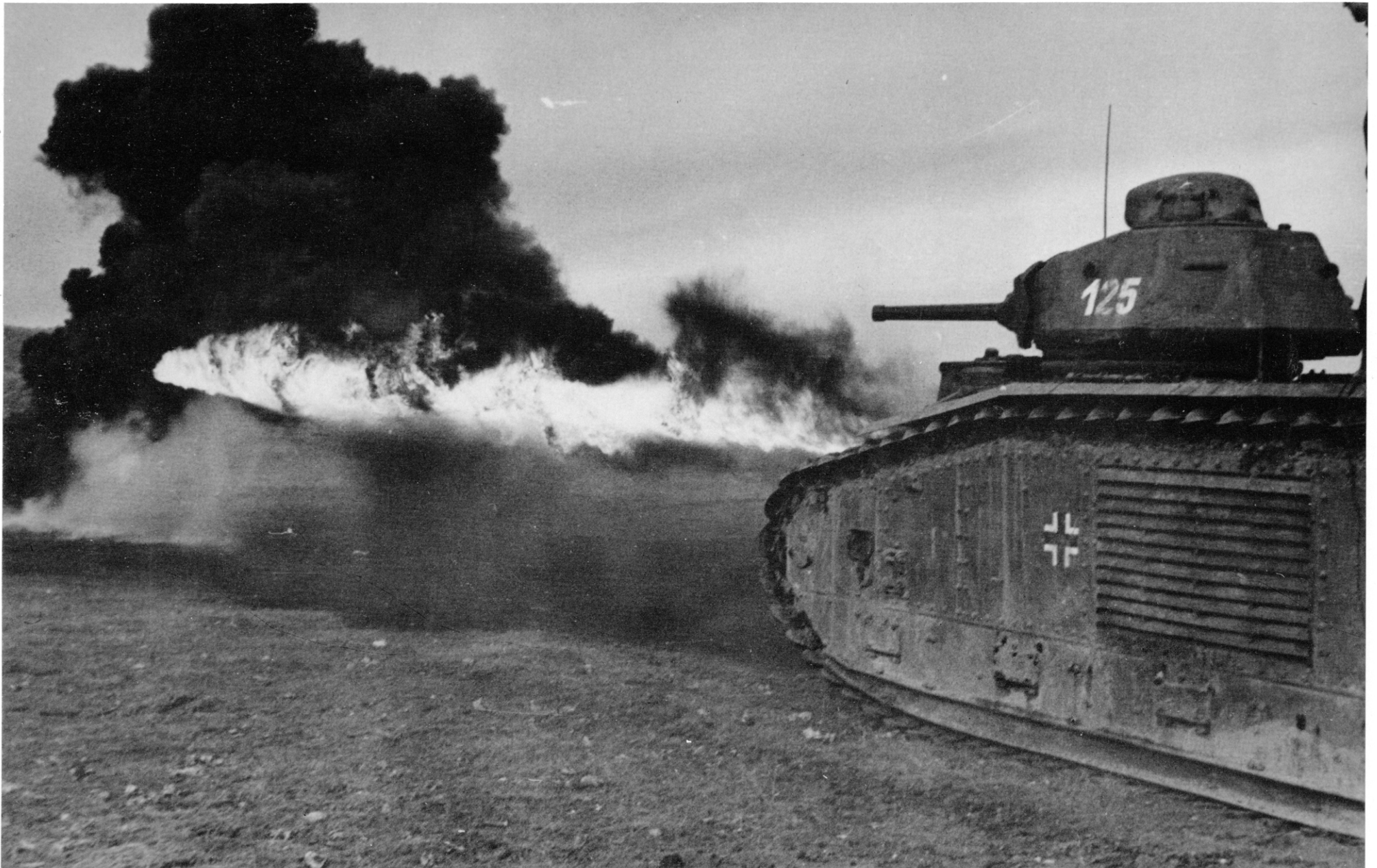
Some of the heavy "Char B1" tanks captured in France were also rebuilt and used as flamethrowing tanks. The 75 mm howitzer at the front of the tank was replaced by a flamethrower. (BA)
