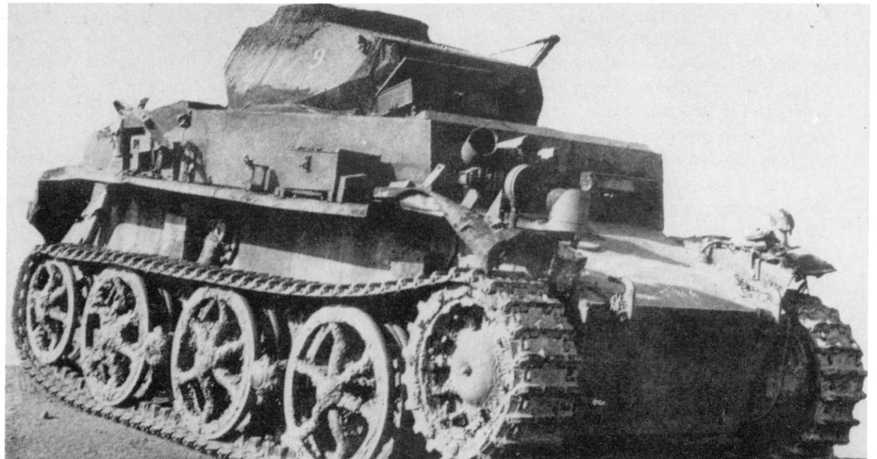
Numerous VK 601 were lost in action in Normandy, and some of them were captured by the Allies. The road wheels of the first series of the box running gear are missing, as is the armament from the turret. Note also the launchers for smoke bombs, mounted on the track aprons in this type of vehicle. (RAC)
