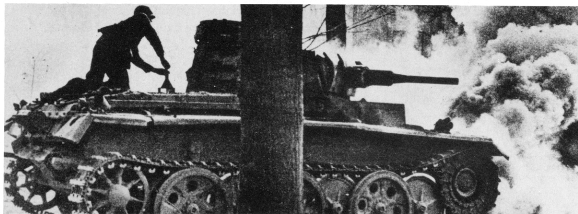
The few Panzer III chassis with Famo box running gear were used almost exclusively for training purposes at various troop training bases. The lower picture shows practice in attaching a hollow charge to the engine compartment of a tank. The prototypes had the same turret as the Panzer III Type J, with the short 50 mm KwK L/42 (2 x IWM)
