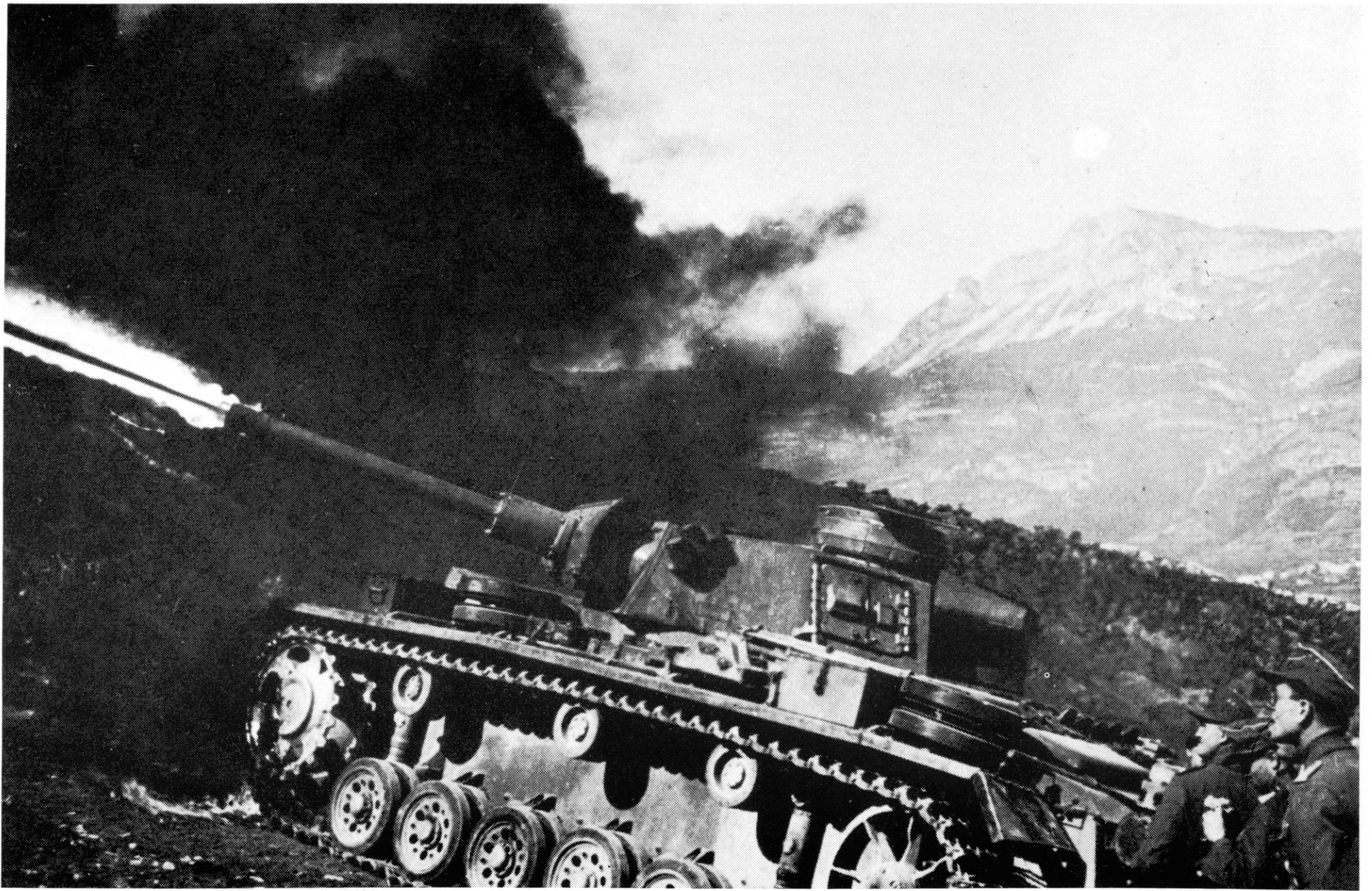
Here a Flammpanzer III of the 44th Infantry Division is seen. The burning oil capacity of 1,020 liters allowed eighty bursts of flame, each two to three seconds long. These vehicles, though, did not live up to the troops' expectations. For that reason, some of the Flammpanzer III tanks were soon (1943) rebuilt into normal battle tanks.
