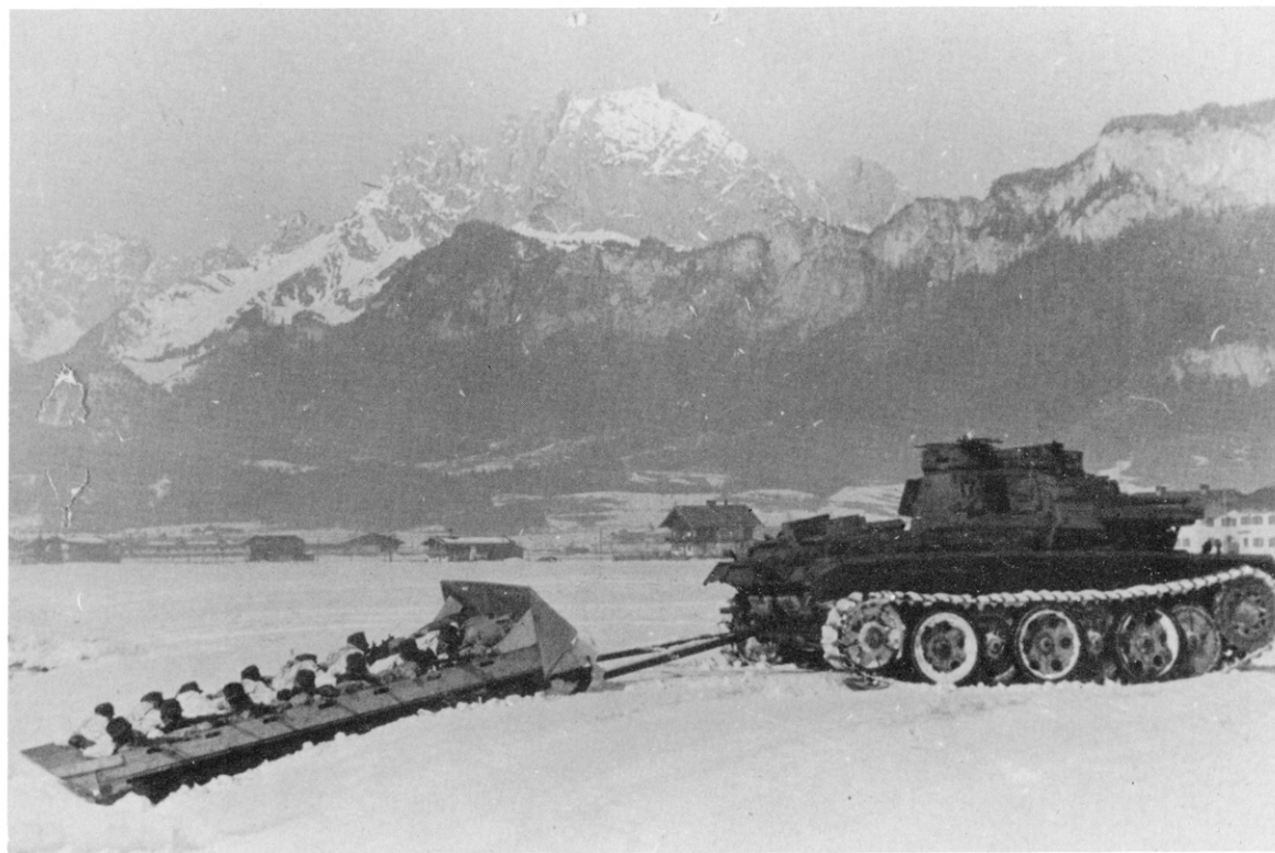
The Panzer III with Famo running gear was also used for testing purposes, as seen here in the winter of 1943, to test the tank trailer sled built by the Ambi.-Budd.-Werke. This device was connected to the tank by a towbar three meters long. It was meant to provide effective infantry support for the tank in the winter conditions of Russia. This project too, sensibly, never went into production. (3 x BA)
