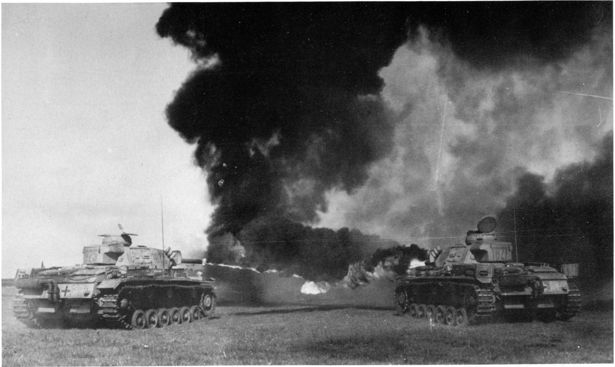
Two Flammpanzer III at a troop training center. The four-digit numbers on the turret can no longer be identified. The burning oil carried inside the tank was directed into the pipe by a pump and there ignited by high-tension electricity (1,000 V, 300 A). The flamethrower was operated, via foot pedals, by the tank commander, who also had to operate the machine gun, elevation apparatus and turret turning apparatus. The flamethrowing pipe had a field of elevation from +20 to -10 degrees. Thus, targets of varying heights and ranges could be attacked. After every burst of fire, though, the air was so full of smoke that the day was turned to night and new targets could scarcely be seen. (BA)
