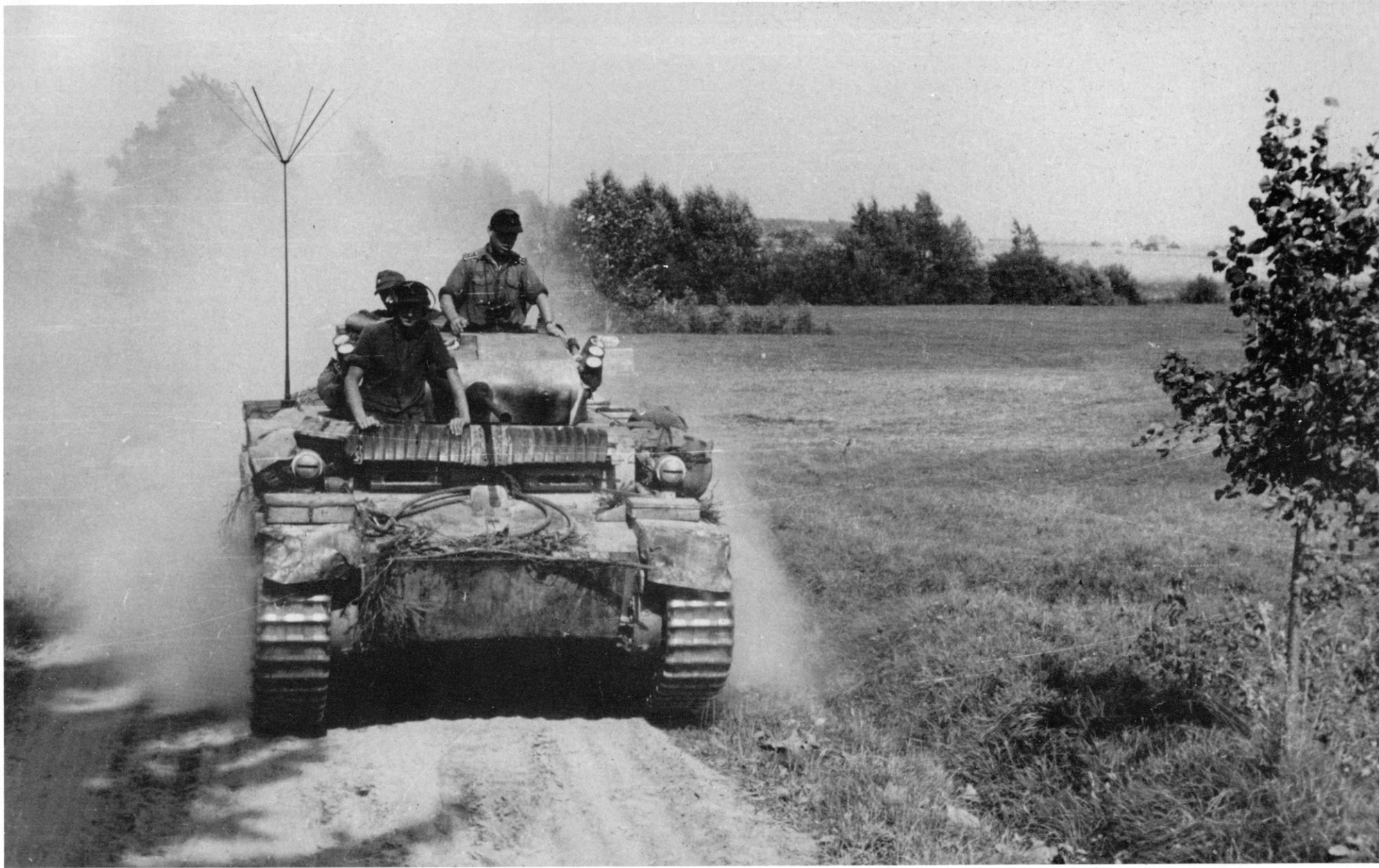
One of the extremely rare action photos of the "Luchs". It was used almost exclusively in Russia. The design of this tank had been made with the extreme climatic conditions of Russia in mind. Thus, it had a cooling-water exchanger that allowed it to be filled with already warmed cooling fluid from other vehicles when the outdoor temperatures were low. The armor plate, with a maximum thickness of 30 mm, was extremely meager. For extra protection, pieces of a Russian tank's tracks have been added above the driver's visor on the hull, just below the bottom of the turret. (BA)
