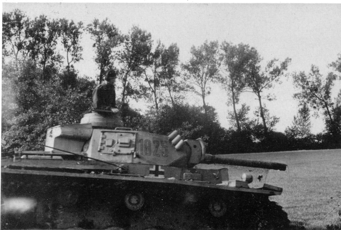
The flamethrowing tank most widely used by the troops was the Flammpanzer III. It carried 1,020 liters of inflammable oil in two containers, which were installed inside the tank. The three smoke-cartridge launchers attached to the turret walls can be seen clearly here. Almost every armored unit had a platoon with five flamethrowing tanks. (BA)
