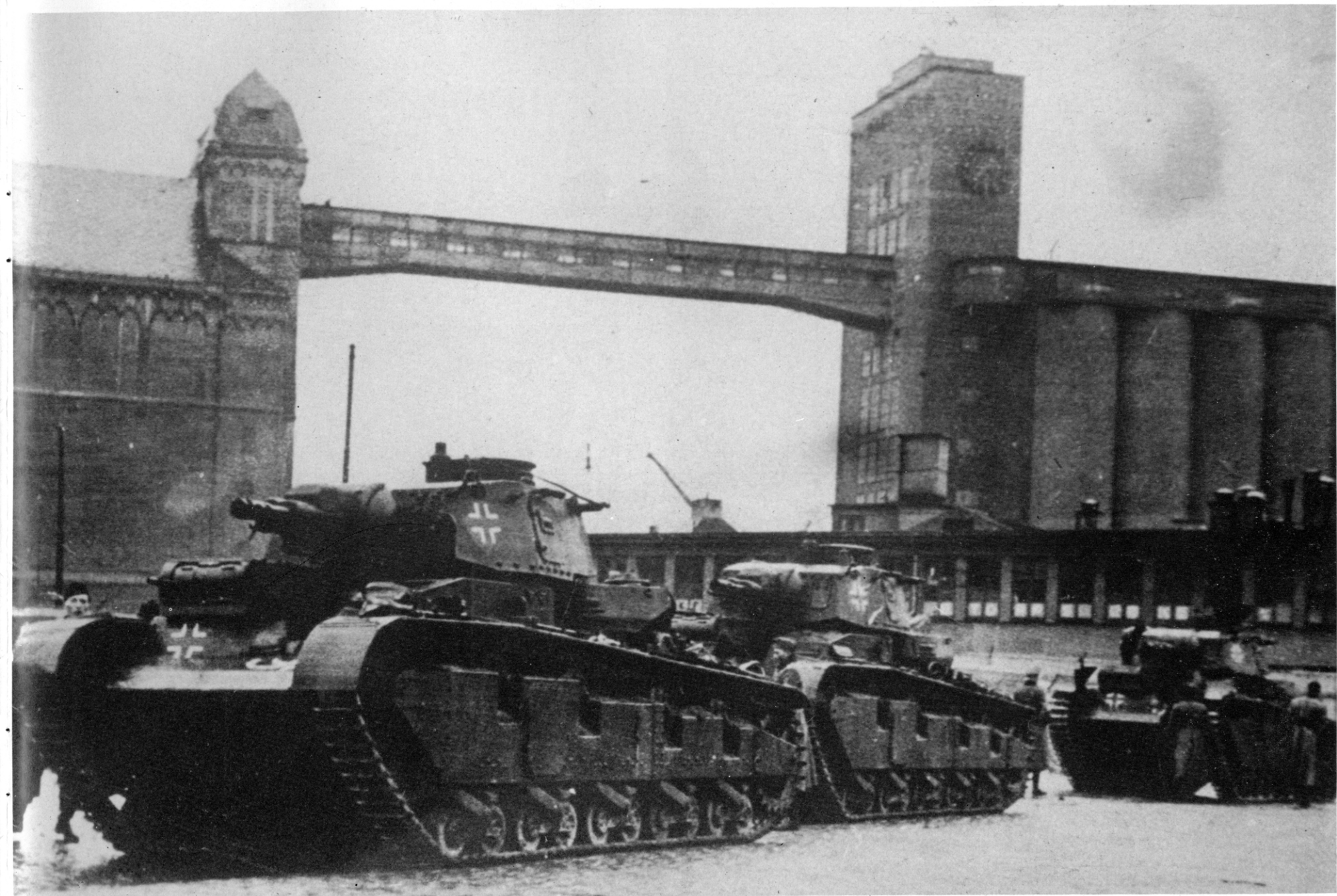
This picture shows all three vehicles shortly after being shipped out. They were supposed to make it look as if large numbers of heavy tanks were available, and thus were often displayed. Because of their light armor plate (13 to 20 mm), though, the combat value of these vehicles was meager.
