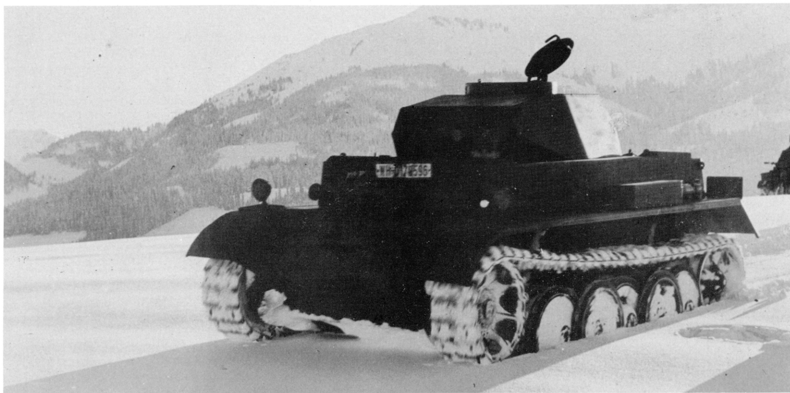
This picture shows the VK 1301 already fitted with the planned turret, but as yet without weapons. (BA)
