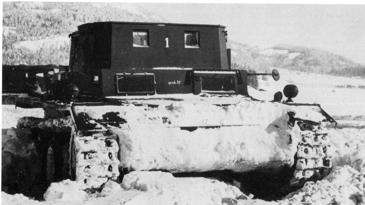
Above: A picture of the only completed VK 1301, including turning turret with full armament. (BA)
