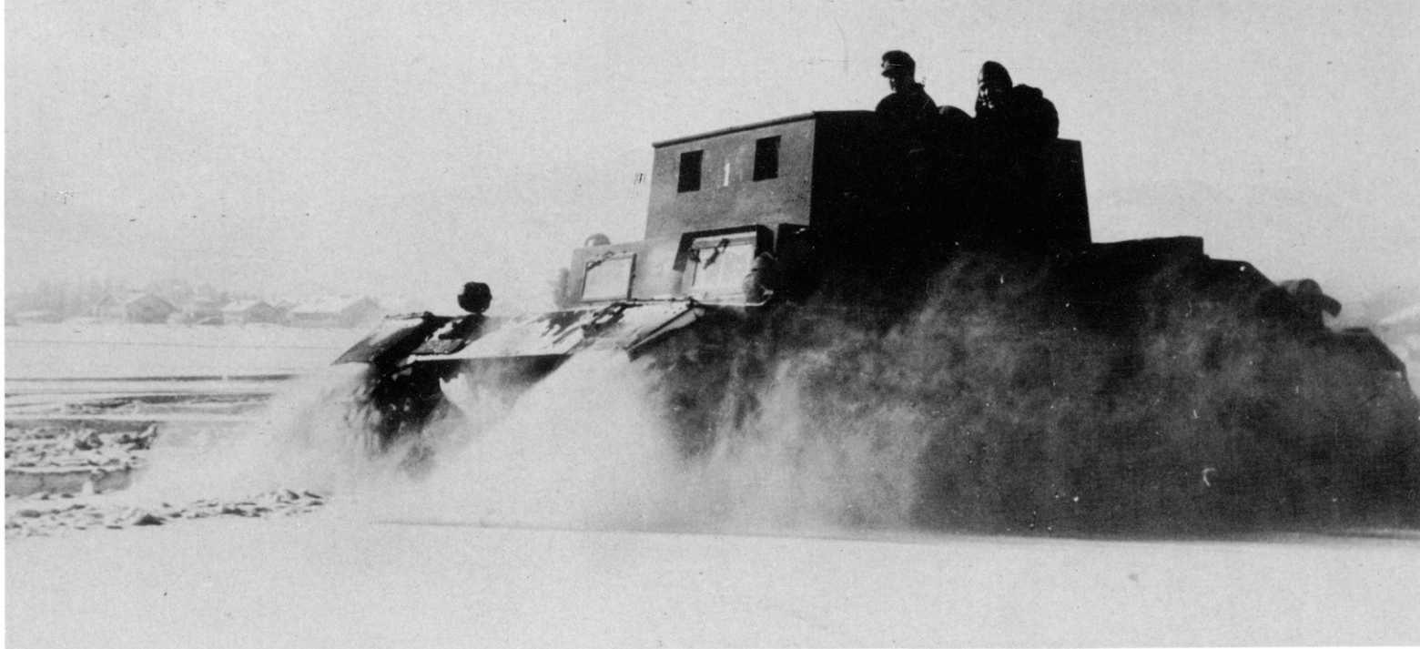
This VK 1301 charges over the deep snow of the terrain at top speed. The exhaust system of the tank was mounted at the rear, and can be seen here. (BA)
