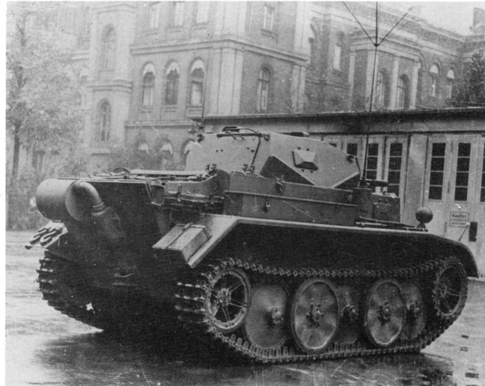
Above: This view gives a good impression of the layout of the vehicle. The entire rear section was taken up by the engine, whose air-intake and ventilation openings, protected with grids, can be seen clearly. The body, unlike that of the VK 1301, extended out over the hull so it could hold the newly designed turret. (RAC)
