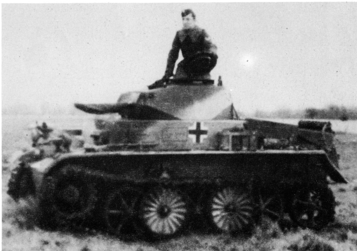
One of the few action photos of the VK 601, probably taken during the Allied invasion of Normandy. The vehicle had a two-man crew. The driver was housed in the right side of the hull, and the commander sat directly behind him in the turret. He could observe his surroundings through eight periscopes (Kinon blocks) arranged in a circle in the cupola. (IWM)
